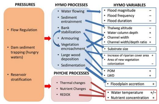
Figure 3.- Conceptual frame work of large dams and reservoirs effects on Hydromorphological (HYMO) and Physic-Chemical (PHYCHE) processes and variables (POM=Particulate Organic Matter; LWD=Large Woody Debris).
