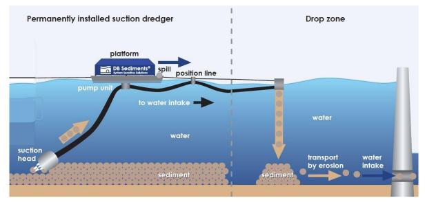
Figure 8.- Hydraulic pumping system to remove accumulated sediments from reservoir tails into the bottom outlet of the dam, in order to be flushed downstream the dam (Bartelt et al. 2012).
